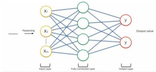
Gambar 6 Contoh Proses *Fully Connected*
