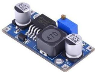
Gambar Error! No text of specified style in document..4 Modul Step Down
