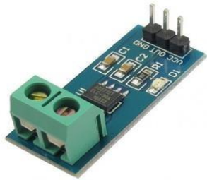
Gambar Error! No text of specified style in document..3 Modul ACS 712 30A
