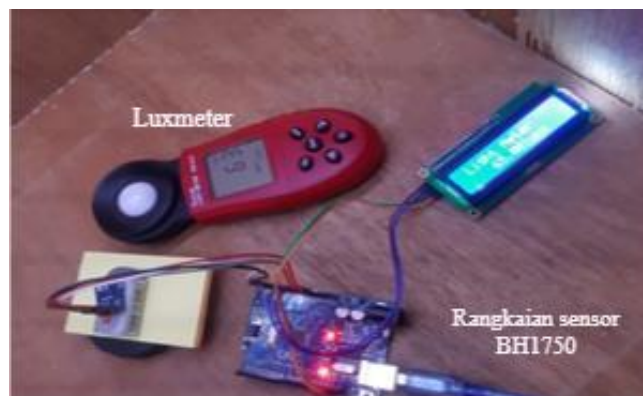
Gambar 4. 6. Proses kalibrasi sensor BH1750
