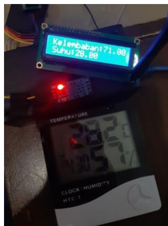
Gambar 4. 3. Proses kalibrasi sensor DHT11
