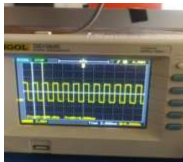
Gambar 3.1 Sinyal PWM 50% Duty Cycle
