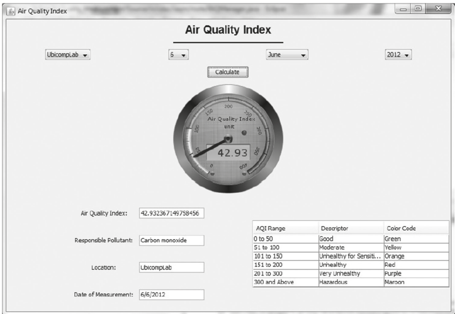
FIGURE 4.7 Air quality index monitoring system [84].
