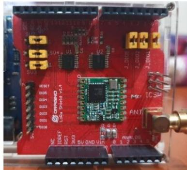
**Gambar 2.2** LoRa Arduino Shield
