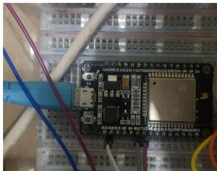
**Gambar 2.5** Modul ESP32
