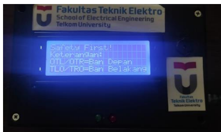
Gambar IV-7 Alat Pengukur Tekanan Ban TG105
