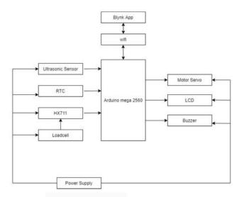
Figure 10 Block Diagram
