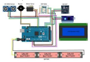
Figure 12 Pet Feeder System Circuit Schematic
