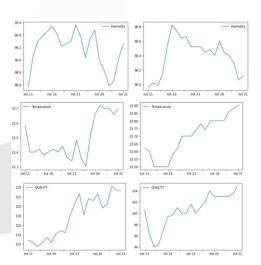
With this test, the only result difference is in the quality of data reading by almost 20 PPM, and at the humidity and temperature, there is not much of a differ- ence. The measurement test will use configuration 2 as the main way to read the data because configuration 1 is often caught by the propeller if not secured properly, and it has a much slower air velocity.
