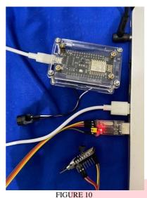
ESP32 CAM AND NODE MCU PUT TOLAPTOP
