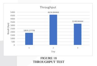
In throughput testing using a WiFi network, on the first day the results were 1859.27 bp/s. On the second day, the result was 4634.84 bp/s, and on the third day, the result was 3248.37 bp/s. From the results of the throughput test for 3 days, the value obtained is in the very good category, according to the ITU-T G1010 standard. The throughput results
