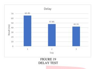
In the Delay test using a Wi-Fi network, on the first day the results were 65.95 ms. On the second day, the result was 47.85 ms, and on the third day, the result was 42.31 ms. From the results of the delay test for 3 days, the value obtained is in the very good category, according to the ITU-T G1010 standard. Throughput results are variable and can be caused by network quality, and protocol performance which takes time to process posts and requests between the device and the server.
