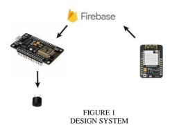
This chapter will discuss the design of a smart parking system tool, this system is equipped with an Esp32 Cam which functions to integrate the presence of vehicles through an integrated video camera. Esp32 cam retrieves data using the image classification Yolov3 method, then the data will be sent through the firebase database in real-time, after which the Node MCU will receive data from the firebase and issue an output in the form of a buzzer.
