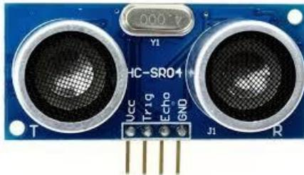
Gambar 3 Sensor Ultrasonik HC – SR04
