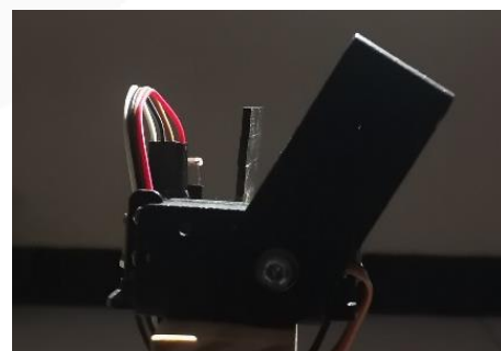
Gambar 4 – 6 Arah Pengujian Servo 135°
