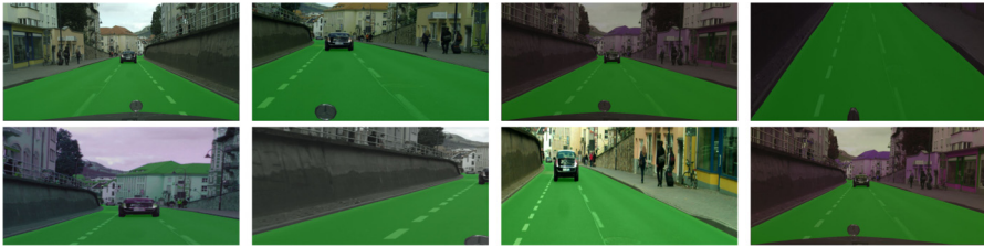
Fig. 1. Seven possible Color-Flip-Crop augmentations on a random training sample. The original sample is on the top-left. We show ground truth mask for illustration purposes, they are not used during training.
