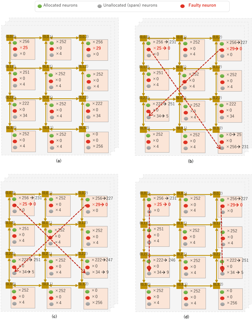
Fig. 8.11 Illustration of fault-tolerance remapping of the Genetic Algorithm. (a) Unmapped and free neurons per node. (b) A randomized mapping solution. (c) Mutating by finding a shorter distance for a flow; (d) Mutate by swapping destination of a flow
