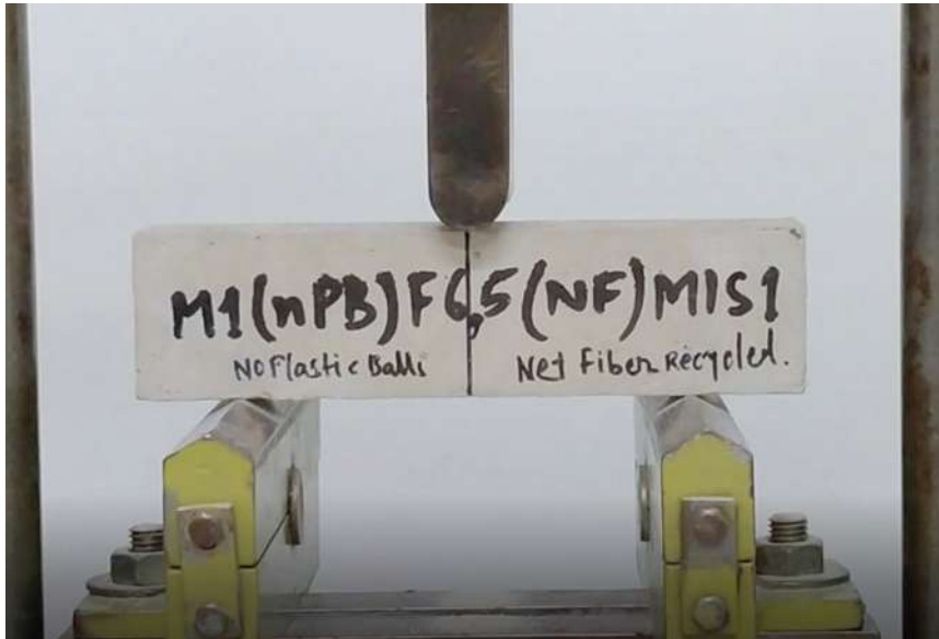
Fig. 5. Flexural strength test
