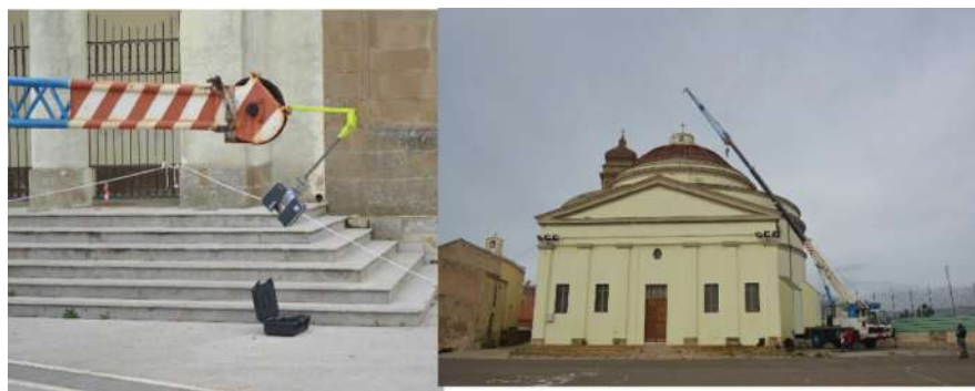
Fig. 3. TLS survey of the roof
