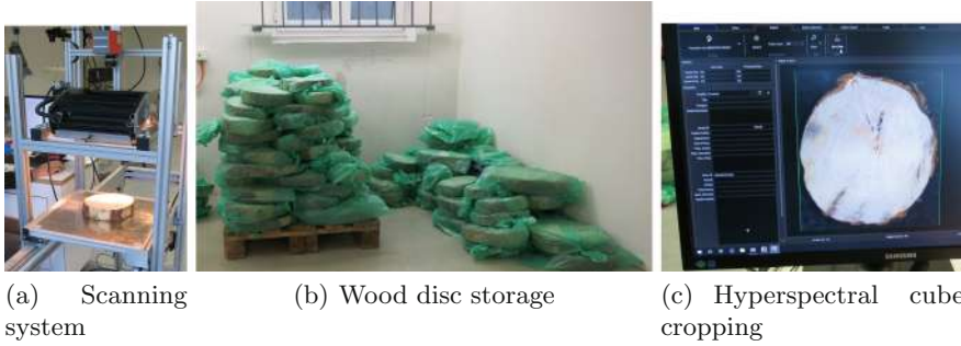
Fig. 1. The sensor system shows the line scanner which was mounted on a metal frame and the slice is moved perpendicular to the scanned line manually. The stored samples were closed airtight to avoid surface changes. Each hyperspectral cube was cropped to reduce the massive amount of data.
