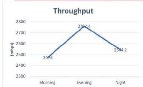
Figure 16 ESP8266 and website application throughput test graphs
