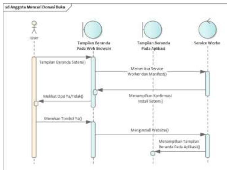
**Gambar 6. Sequence Diagram : Install ELIT ITTelkom Surabaya**
