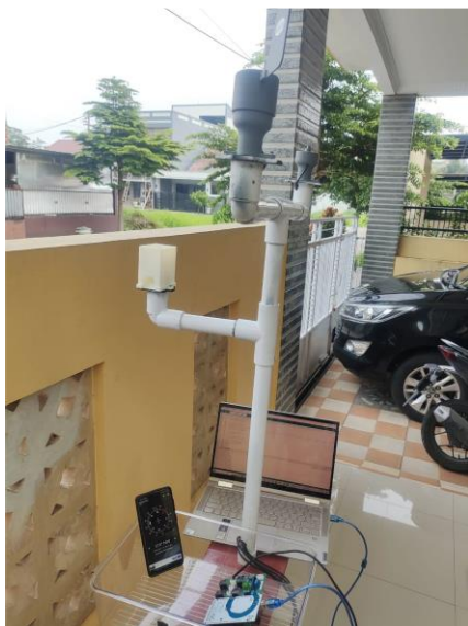
Figure 13 Wind Vane Direction Testing
