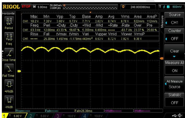
Gambar 4.3 Hasil pengujian Three Phase Rectifier tanpa kapasitor
