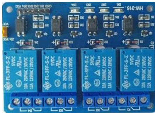
**Gambar 4. 19 Relay 4 Channel**
