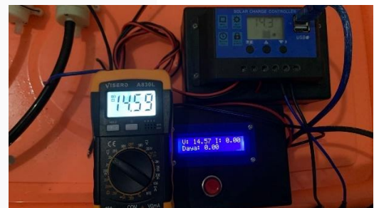
GAMBAR 15 Rangkaian Monitoring Baterai
