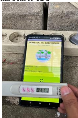
GAMBAR 12 Pengujian Sensor TDS
