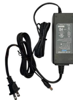
Gambar 6 (Power Supply 12 V 3 A)
