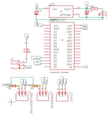
GAMBAR 4 (Wiring Schematic)
