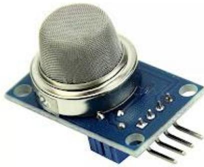
Gambar 3 sensor gas MQ-2
