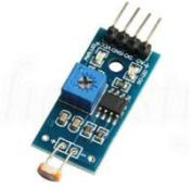
Gambar 2 MH Photoresistor Light Sensor Module
