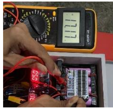
Gambar 13 Rangkaian Baterai 4S 2 paralel, 4 series
