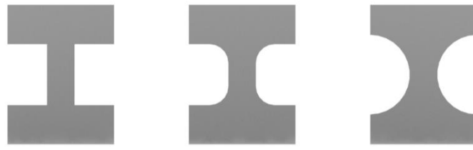
Gambar I. 3 Tipe flexure hinge , (a) leaf spring hinge , (b) corner-filletted hinge , (c) notch hinge (Dimodifikasi, dari, (Linß et al., 2017) © Copernicus)
