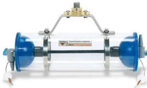
Gambar 1. 1 Water Sampler (Kemmerer)
