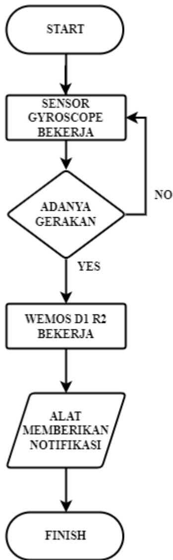
Gambar 3 4 Flowchart Sensor Gyroscope
