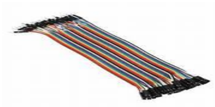
Gambar 2 5 Kabel Jumper Male – To – Female
