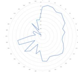
Figure 4.6 6 GHz Azimuth Radiation Pattern.
