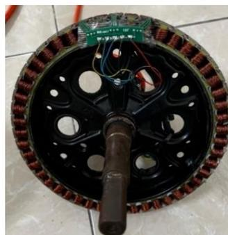
**Gambar II. 10 Stator BLDC**
