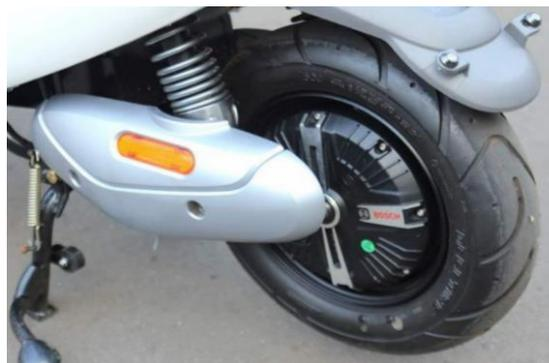
*Gambar II. 7 Motor Motor Wheelhub*
