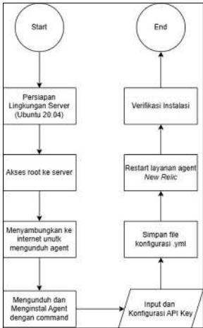
GAMBAR 2 Flowchart Instalasi Monitoring Agent New Relic
