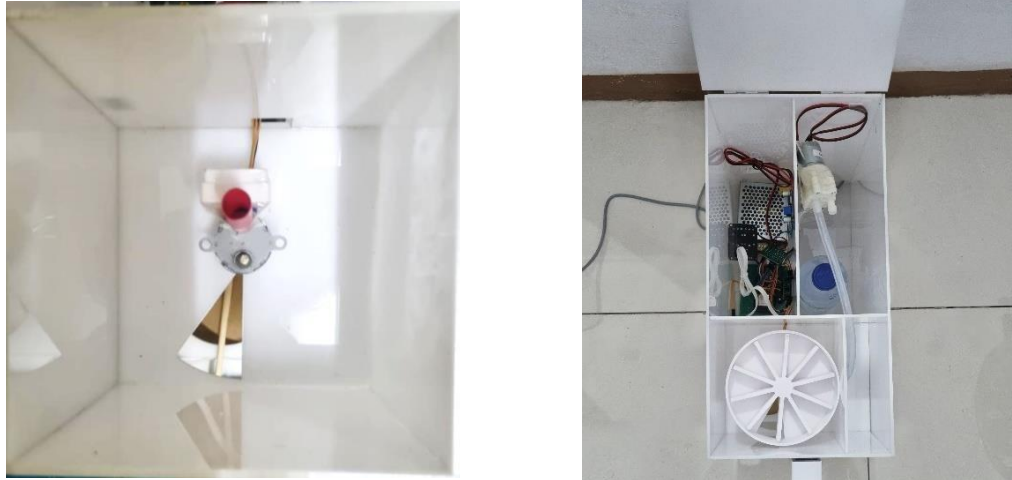
Gambar 5. 3 Gambar Implementasi Motor Stepper dan Water Pump
