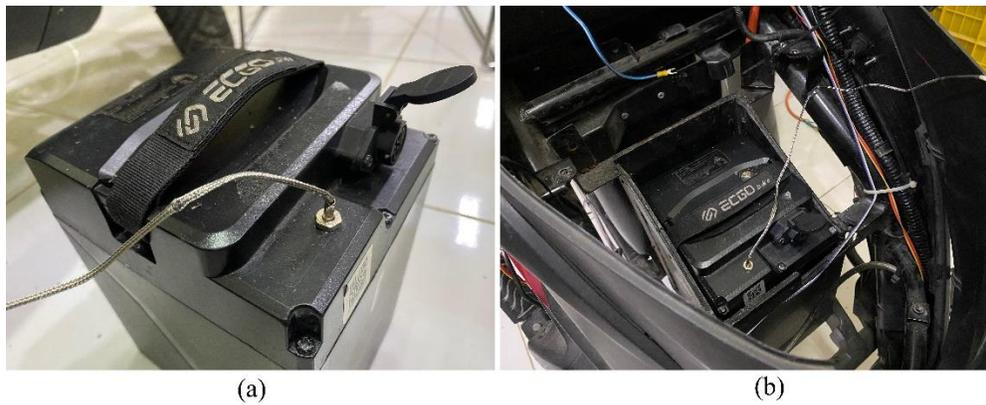
**Figure 3. 6** (a) Temperature Sensor Position, (b) Battery Position
