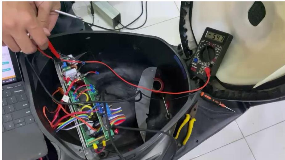
**Figure 4. 3** *Voltage Check of the System with Step-up*
