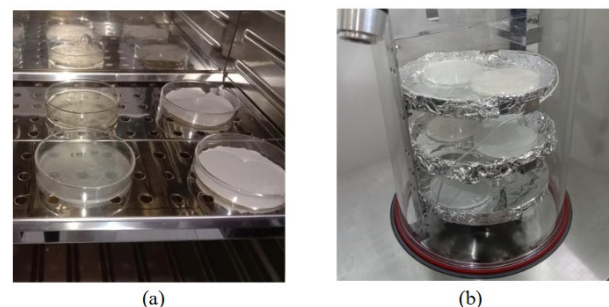
GAMBAR 3 (PROSES PENGERINGAN; (A) OVEN-DRYING (B) FREEZE-DRYING)
