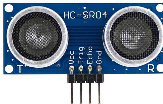
Gambar 2.2 Sensor Ultrasonik
