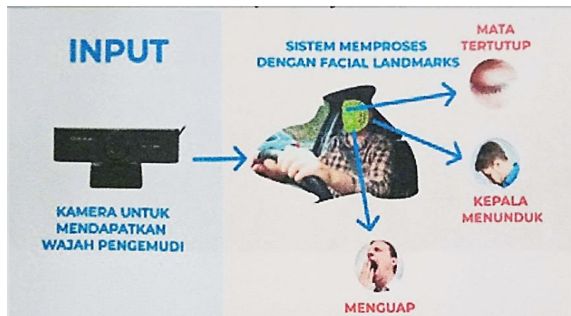
Gambar 1.5 Cara Kerja Teknologi Driver Assistance
