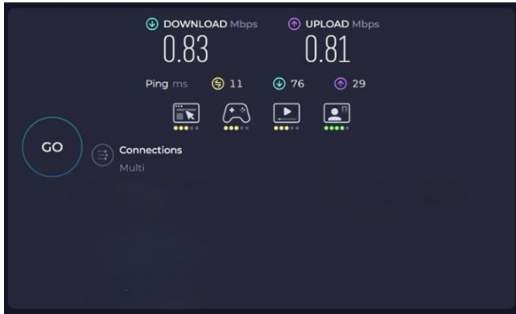
Gambar 5.16 Speed test jaringan RT/RW Net.
