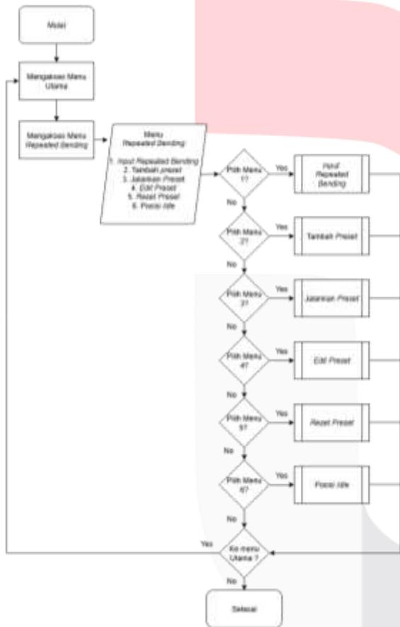
Gambar 3 *Flowchart* Alur Pengujian *Repeated Bending*.
