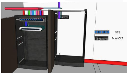
Gambar 3 Drafting jalur fiber optic
