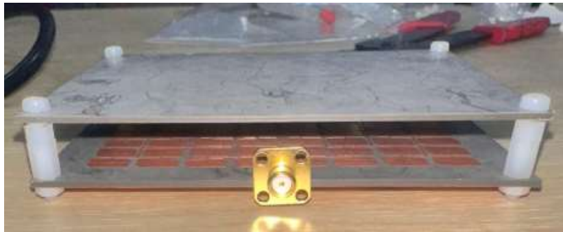
Figure 4.3 Fabricated 64-Element Antenna Array with Integrated Metamaterial.
