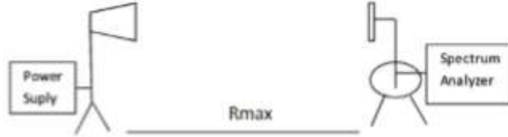
Figure 4.6 Antenna Arrangement for Radiation Pattern Measurement.
