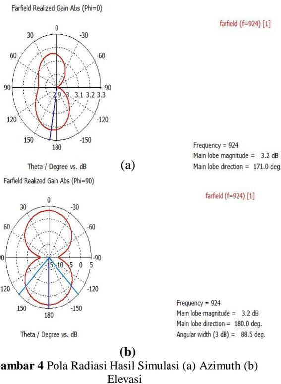
**Gambar 4** Pola Radiasi Hasil Simulasi (a) Azimuth (b) Elevasi
