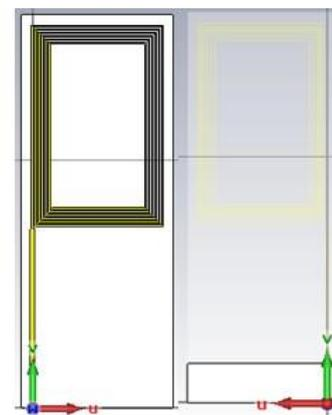
Gambar 2 Desain Antena Mikrostrip Rectangular Monopole Spiral
