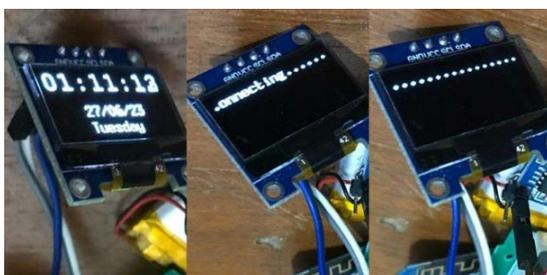
Gambar 8. Layar OLED *Smartwatch*
